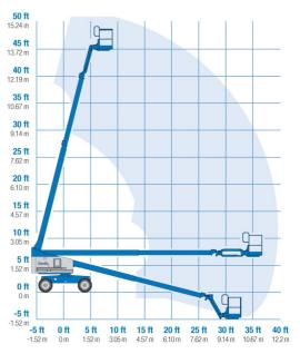
\* The metric equivalent of working height adds 2 m to platform height. U.S. adds 6 ft to platform height.
